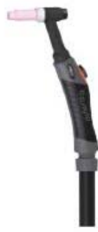
TIG torch: DGT 26 Cooling Method: Air-Cooled Rating: DC 200A AC 125A Duty Cycle: 35% Electrode Size: 1.0-4.0
